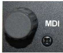
Selects Altitude Alert/Decision Altitude on Radar Altimeter (King Air B200)
