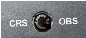
Switches between HSI and OBS #1
