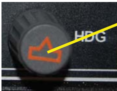
Selects the heading using the heading bug
